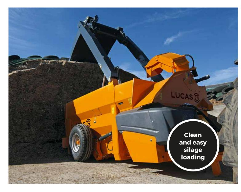
The range of silage feeders Castor G is composed of four models from 4 to 8 m<sup>3</sup> capacity. These machines are equipped with rounded claw to unload the silage and ensure a simple and clean load of silage, once loaded the distribution is made by the turbine. The silage unloader Castor G can be fitted with a mixing hopper for dry food.
