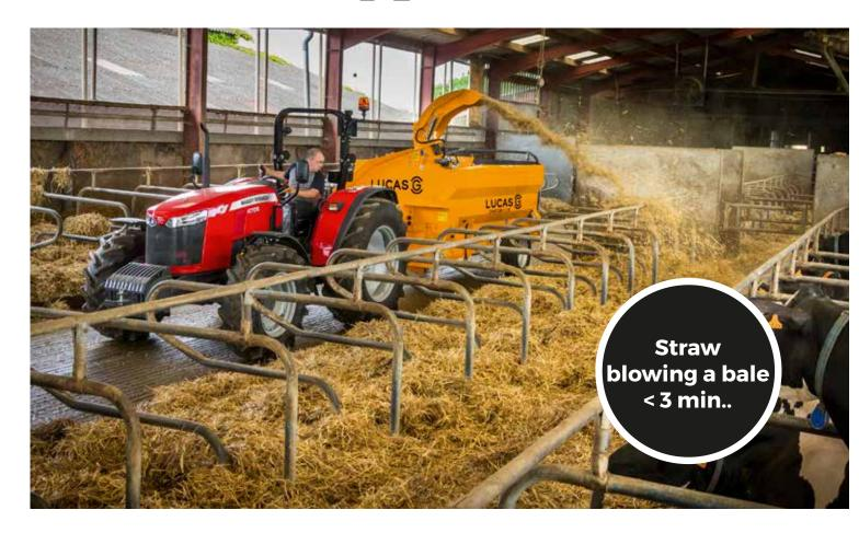
The range of bale feeders Castor R is composed of seven models from 2 to 18 m<sup>3</sup>. These straw blowers are equipped with 1, 2 or 3 mechanical shredders, depending on their capacities. The main benefits of these bale feeders are that they have been designed to distribute all type of material, corn silage, grass, alfalfa, regardless the size of strand (short or long) and the degree of humidity.
