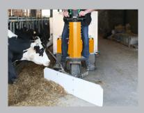
Fodder pusher blade To push back the ration while distributing the concentrates. Lifting is manual
