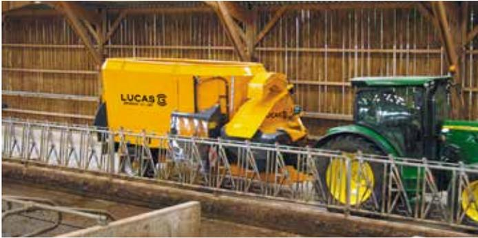
The SPIRMIX feeders are designed for intensive and daily use. These mixers are adaptable depending on the configuration of the farm and the type of livestock. The machines feature a heavy-duty construction and independent axle for better towing characteristics increased longevity.
