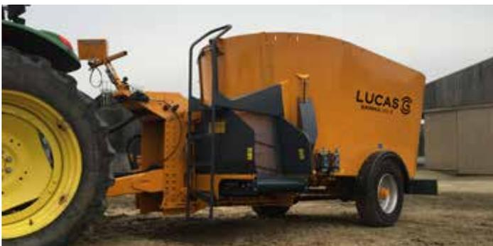
The SPIRMIX S diet feeders have been developed for farms where machine size is an important factor. These machines are compact and manoeuvrable. The rear axle is positioned to provide a very low overall height without compromising manoeuvrability. The lowered machines are ideal for farms where the layout of buildings has height restrictions.
