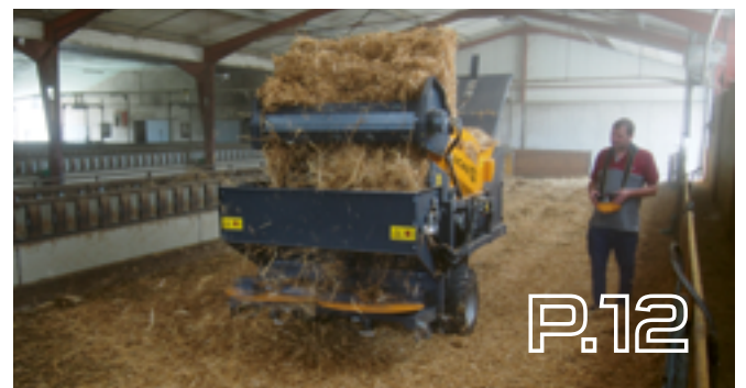
UBI SWITCH Versatile remote controlled bale unroller
